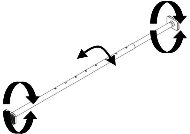
Twist the end pads until they touch the sides of the cargo area. Then twist the bar to tighten. Tighten the cargo bar until the cargo is secure. **Be careful not to over tighten the cargo bar, as it can cause damage to the cargo area.**
