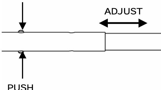
To adjust the bar, depress the pushpins and slide the bar in and out to the closest width.
