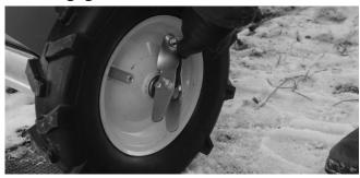
NOTE: If you will be making a large number of turns while spreading engage only one wheel. Engage the wheel opposite of the way you will be turning. For example, if you're turning right engage the left wheel. For straight line spreading or heavy loads, engage both wheels. Optimal speed for best results are between 10-16 mph.
