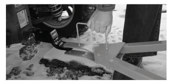
2. Once holes are aligned, drop in the hitch pin.
