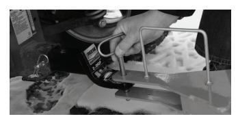
3. After the hitch pin has been successfully placed through the hitch and tongue, then install cotter pin.
