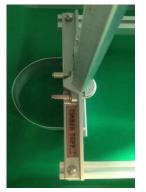
With the guard assembly attached to the frame bracket and long rails, adjust to desired cutting thickness (minimum 3 inches) and tighten nuts around U-Bolt.
