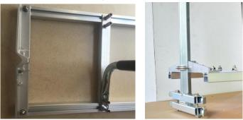
With the end post assembly attached to the frame bracket and long rails, adjust to desired cutting thickness (minimum 3 inches) and tighten nuts around U-Bolt.
