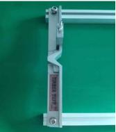
7. Attach chain guard assembly to the frame bracket (#6) using U-Bolt (#9), U-Bolt Adaptor/Clamp (#10), washers (#11), and long hex nuts (#2).
