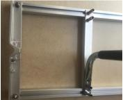
5. Assemble the end post (#7) to bottom bracket (#8) using long bolts (#12) and washers (#11).
