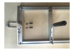
7. With the sawmill assembled, set the desired cutting thickness (minimum 3 inches) and tighten nuts around the U-Bolt.
