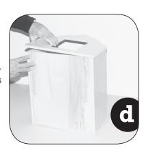
Using the provided screws, screw the end panel through the pre-drilled holes onto the side panels.
