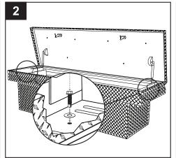
2. On each end of the tool box, secure with 3/8 in. self-tapping sheet metal screw and 3/8 in. fender washer in top lip of tool box, 1 in. from end of box. Screws should be securely anchored through box into bed rail of truck.
