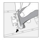
STEP 2: Lift accessory out of slot at angle to remove.
