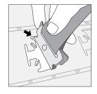
Press locking lever and push toward locking lever end of slot.
