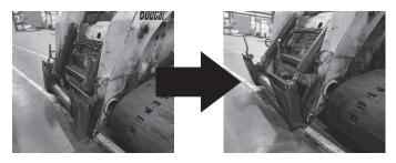
2. Drive the loader forward slowly making sure the top edge of the attachment plate is completely under the top flange of the snow pusher mounting frame. Then tilt the attachment plate backward.
