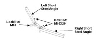
Connect the Front Steel Angle Assembly to the Rear Steel Angle
