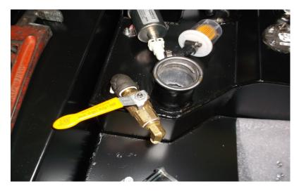
The orientation of the supply hose and valve going to the refueling pump may be changed to fit the customers preference. Make sure the supply line the pump does not kink.
