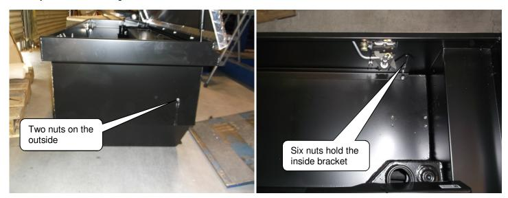
3. Once you have the height set and confirmed tighten the 5/16 flange nuts using the torque specs in IS #484 to make the toolbox stationary on the tank. Take a measurement from the ground to the knock outs to be used comparing to the measurements you took earlier.
