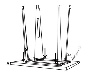
1. Attach each Table Leg (C) to Table Top Frame (A) using 8 pieces screws (D).
