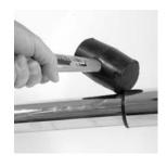
To remove the Table Top from the Support Cylinder, turn the table upside down, and strike the edge of the Support Cylinder several times where it meets the support leg of the tabletop. The Support Cylinder and Table Plate and Leg will separate with applied force.
