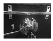
**1**. Use a hex wrench to attach the Support Cylinder (C) to the underside of the Seat (F) with the provided hex bolts.
