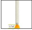
Optimal stickout varies by electrode type and diameter but is approximately 1/16"
