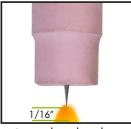
Optimal arc length varies by electrode type and diameter but is approximately 1/16"
