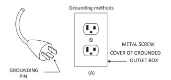
This appliance is for use on a nominal 115V circuit, and has a grounding plug that looks like the plug illustrated in sketch A. Make sure that the appliance is connected to an outlet having the same configuration as the plug. No adaptor should be used with this appliance.
