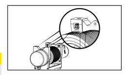
Place the mounting plate on the winch, making sure the winch is centered in the middle of the mounting plate.
