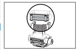
Attach using the 4 M10 cap screws with 4 lock washers and flat washers into the hole.
