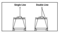
This reduces the load on the winch and the strain on the rope by approximately 50%.
