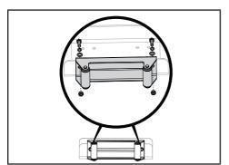
2. Turn the winch up-side-down; insert 4 M10 nuts into the holes of the winch.
