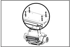
Turn winch right side up. Disengage the clutch by moving the cam ring to the "Out" position. Release the rope and pull through the roller fairlead.
