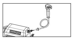
4. Check for proper drum rotation. Pull and turn the clutch knob to the "out" position (Free spooling). Pull out some cable from the drum, and then turn the clutch knob to the "In" position to engage the gears. Press the cable out button on the handlebar switch. If the drum is turning and releasing more cable then your connections are accurate. If the drum is turning and collecting more cable then reverse the leads on the motor. Repeat and check rotation.
