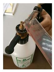
1.2 In this case if you were to set the dial to number 1 you would be the mixing 3ml of insecticide or fertilizer per liter of water. Similarly, if so set the dial to number 2 you would be mixing 6ml per liter of water. The chart below sets out the concentrations:
