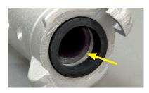
After installing the coupling / nozzle holder, check that the blast hose is flush against the coupling all the way around verifying it has been cut square and inserted completely.
