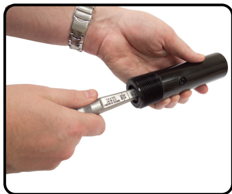
STEP 3: Insert the gauge into the threaded/inlet side of the nozzle until it stops and give it a couple of turns.
