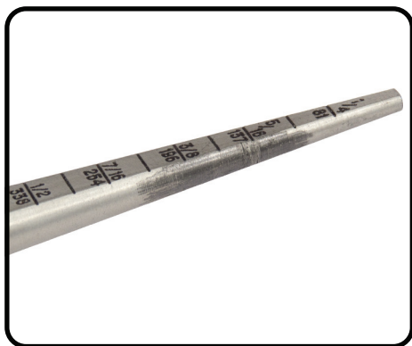
STEP 4: Remove the gauge and locate the mark closest to the handle where the nozzle rubbed off the marking pencil/crayon. This is the current ID of the nozzle bore.
