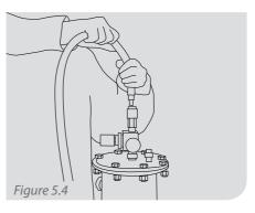
Connect the Air Supply Hose Tail to the point of attachment supplying Grade D air.
