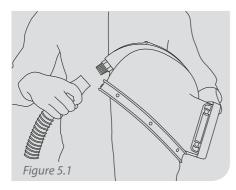
First screw on the breathing hose in a clockwise direction onto the helmet.
