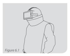
Once the helmet is fitting comfortably on your head, straighten the cape down at the front and back.
