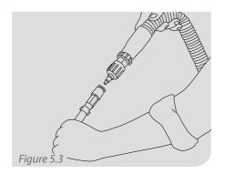
Take the quick dis-connect fitting on the Air Supply Hose and push onto the tail of the Flow Control Device.
