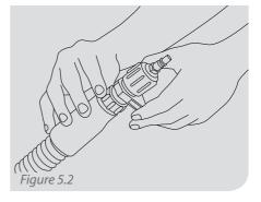
Screw the loose running nut in a clockwise direction onto the flow control device (2016).
