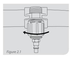
Air flowing into the helmet is controlled using the regulator as shown in Fig 2.1 and 2.2.
