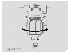
**NOTE:** The minimum of 170 Vmin should be flowing through the helmet when the regulator is in the closed position as in Fig 2.2 and the pressure set in accordance with the table on page 8.
