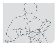
Make sure the window frame gasket is securely fitted in the helmet with no cracks or tears in the seal. Check that the inner lens is correctly fitted into the gasket.
