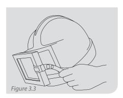
Fold the visor across the front of the helmet and lock the strap tightly over the side cleat.
