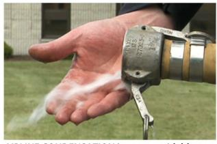
AIRLINE CONDENSATION is an unavoidable byproduct of the air compression process. Condensation occurs when hot & humid compressed air cools in the airline. A 375CFM air compressor operating on a warm humid day will produce more than 30 gallons of water in a single 8 hour shift.
