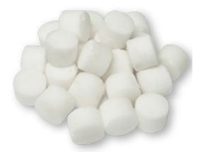
HOW DESICCANT WORKS: Dry-O-Lite® is a dense hygroscopic tablet that absorbs water vapor from streams of compressed air. The surface of the desiccant tablet dissolves slowly, forming a brine solution which drops from the surface. The tablet continuously dissolves, or deliquesces, until the desiccant is fully consumed.
