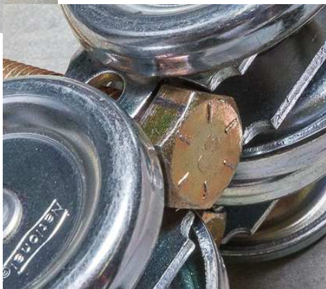
1/2" Bolts shown installed in Roller Assemblies
