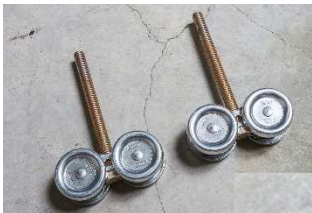
1/2" Bolts shown installed in Roller Assemblies
