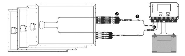
Remove the panel covering. In good sunlight, the charge controller's • "BAT %" should increase to 100%. When the controller is set to "LOAD ON," the system will provide power through the load control output or through the USB port.
