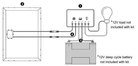
Remove the panel covering. In good sunlight, the charge controller's **0** "BAT %" should increase to 100%. Once the battery is fully charged and the controller is set to "LOAD ON," the system will provide power through the load control output or through the two USB ports. If an inverter is added to the system, it must be connected to the battery bank, and not to the charge controller.
