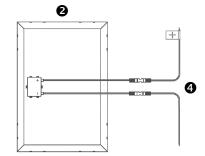
Connect the bare wire end of the positive cable 4 to the "SOLAR +" input of the charge controller 1. Connect the negative bare end to the "SOLAR -" input. Now, you can mount the GS-PWM-20A charge controller to an indoor wall or within a NEMA-3R rated enclosure.
