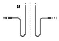
Connect the MC4 ends of the halved cable **4** to the compatible MC4 ends of the solar panel 2 cables. (Mark the end of the positive panel cable with a piece of tape to help distinguish polarity during connection.)
