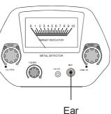
To connect earphones to the detector, insert the earphone's 3.5mm plug into the EAR jack on the control panel.
