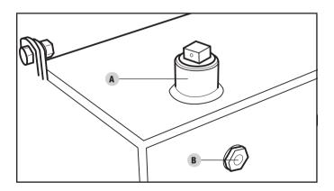
Unscrew and remove the tank fill plug, on top of the tank. Using a funnel add approximately 4 gal. (15.1 L) of hydraulic oil to the tank. Wipe up any spilled oil. (A)
