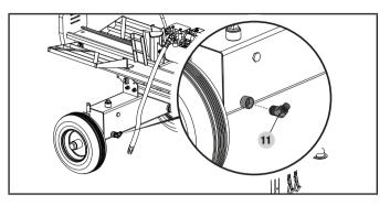
Place an o-ring into tank inlet connector installed in the previous step. Make sure the o-ring is properly placed in the inner groove. Connect the end of hose (19) to the tank inlet connector. Securely tighten the end with a 27mm wrench (Torque: 52 lbf-ft (70.5 Nm) to 66 lbf-ft (89.5 Nm)).
