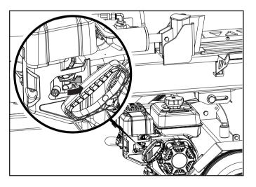
3. Move the choke lever to the "CHOKE" position.
