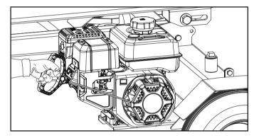
5. As engine warms up, move the choke lever to the "RUN" position.
