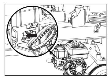
4. Pull the starter cord until resistance is felt and then pull rapidly.
