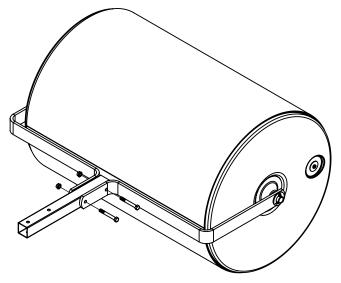
Add clevis bars (4) to hitch tube with 3/8" bolts (5) and 3/8" nuts (6). Install hitch pin (10) and hairpin cotter (11) as shown. 3
