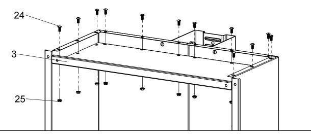
**5** Attach Corners to Body and tighten hardware.
