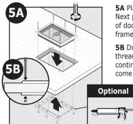
**5A** Place interior frame (frame with flap) into cutout. Next place exterior frame into cutout from underside of door, aligning core covers into tabs of frame. Hold frame together with one hand.
