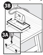
**3A** Drill %" holes in inside corners of drawn template. These will be the pilot holes for the saw blade.
