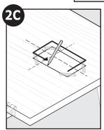
**2C** Cut out the correct template size. Match the marked lines on the door with the shoulder and center lines on the template. Tape the template in place and carefully trace template. Make sure to trace underneath tape and connect the corners. Now, remove the template and any excess tape from the door.
