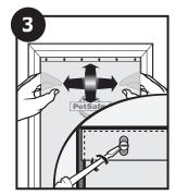
Replace new vinyl flap and position horizontally and vertically to fit into door frame. Replace existing bar and tighten screws in place.
