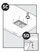
**5C** Use a screwdriver to evenly tighten screws throughout frame while keeping core covers in position. It may be necessary to adjust screws to make sure pet door fit is correct.
