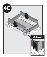
**Optional:** Use duct tape in the corners of core covers to help secure in place and to improve weather resistance. Cut off any excess tape.
