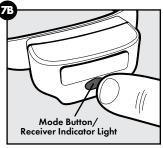
During normal operation, the receiver collar indicator light will flash every 4–5 seconds to indicate the battery status as shown in the following table.
