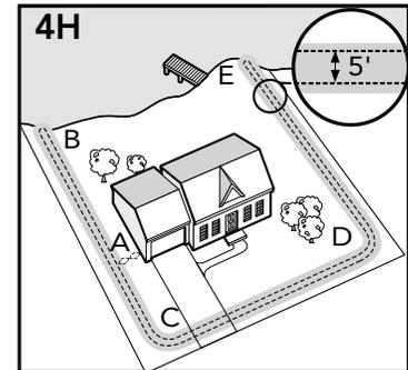
**Sample 5 (4H): Lake Access (Double Loop)** From the Fence Transmitter, run the wire to **A**, **A** to **B**, make a U-turn and go to **C**, **C** to **D**, **D** to **E**, make a U-turn and follow your path all the way back to **A** keeping wire separated **at least 5 feet**. Twist the wire from **A** back to the Fence Transmitter.
