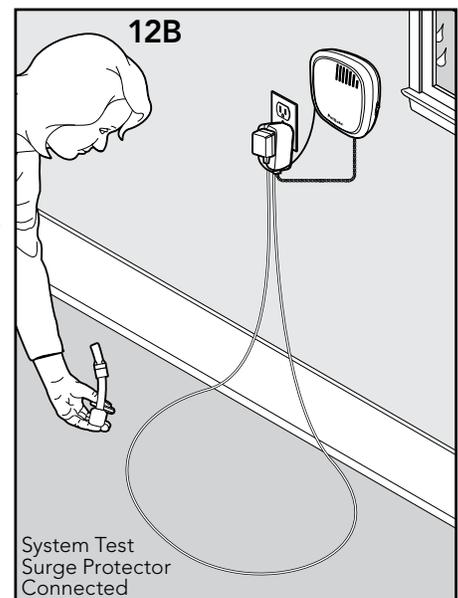
14. When testing is complete reconnect and verify that the Boundary Wire is plugged into the Loop Terminals on the Surge Protector and the Transmitter is connected to the Surge Protector.
