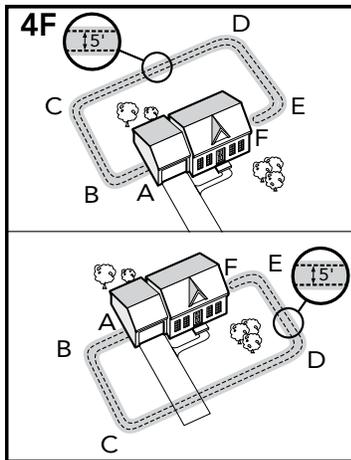
**Sample 3 (4F): Front or Back Yard Only (Double Loop)** From the Fence Transmitter, run the wire to **A**, **A** to **B**, **B** to **C**, **C** to **D**, **D** to **E**, **E** to **F**, make a U-turn and follow your path all the way back to **A**, keeping the wire separated **at least 5 feet**. Twist the wire from **A** back to the Fence Transmitter.
