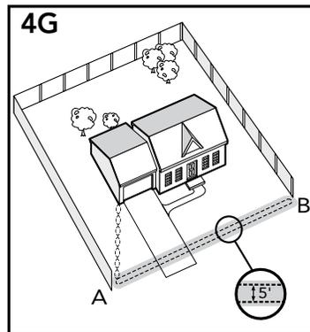
**Sample 4 (4G): Front Boundary Only (Double Loop)** From the Fence Transmitter, run the wire to **A**, **A** to **B**, **B** back to **A** keeping the wire separated **at least 5 feet**. Twist the wire from **A** back to the Fence Transmitter.
