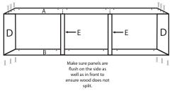
Step 3 Attach Back Panel (C) to both Side Panels (D) and Center Panels (E) using (12) screws (G). Next, attach back panel (C) to Top Panel (A) and Bottom Panel (B) using (12) screws (G).
