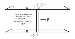
When inserting the center divide for any of the following: Duplex, XL Duplex, or Triplex: Slide Center Panel(s) through grooves to clear any possible debris that may be built up. This ensures the tightest and straightest possible fit.
