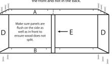
Attach Back Panel (C) to both Side Panels (D) and Center Panel (E) using (9) screws (G). Next, attach back panel (C) to Top Panel (A) and Bottom Panel (B) using (8) screws (G).
