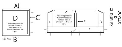
Attach Top Panel (A) to both Side Panels (D) using (6) screws (G). Attach Bottom Panel (B) to both Side Panels (D) using (6) screws (G).
