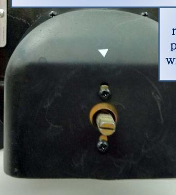
Once valve is removed from fire pit, drill the orifice with a 1/8th drill bit. Reassemble.
