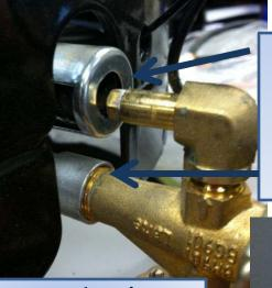
Remove valve from burner, unscrew from thermocouple wire, and disconnect electrode wire.
