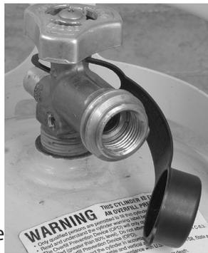
**CAUTION:** In the connection process, the HVR side of the connection will seal on the back check in the valve, resulting in a slight resistance. The connection
