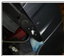
6. Raise hitch into position and secure to frame using 1/2" flange nuts. Secure (2) 10mm bolts and (2) 3/8" conical toothed washers into the existing weldnuts. See WELDNUT CLEANING on page 2.
