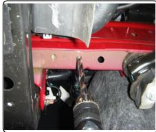
4. Use a die grinder to enlarge (2) mounting locations on vehicle cross member so the included 1/2" hardware can be reverse fishwired into position.
