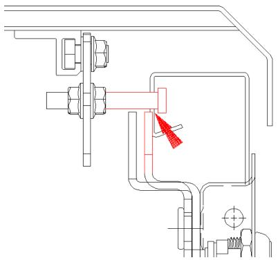
4. Tighten the pin in the lowest location, and close the lid. If the lid is able to move up and down when latched, the latch pin needs adjusted. Adjust the pin up the approximate amount the lid is able to move and retighten.
