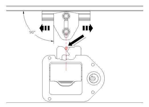
2. When the striker pin is correctly centered, tighten top bolt to set the location.
