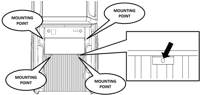
4 Check the underside of the truck bed below the marked locations for clearance. If something is in the way of the marked location, shift the tank to avoid the obstruction.
