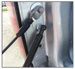
Install the narrow end of the shock on the bottom ball platemount
