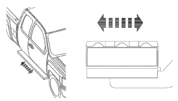
Once the board is in the desired location, tighten the bolts that attach the board to the brace using a 7/16" wrench and socket.
