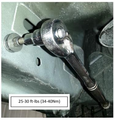
NOTE: ON SOME MODEL YEARS, THERE ARE WELD NUTS INSTALLED IN THE FRONT MOUNTING LOCATION. IF THERE ARE WELD NUTS, THE NUTSERT CAN NOT BE INSTALLED. THE EXISTING WELD NUT WILL BE USED TO INSTALL THE BRACE. INSTALL THE NUTSERTS AT THE MIDDLE AND REAR MOUNTING LOCATIONS.
