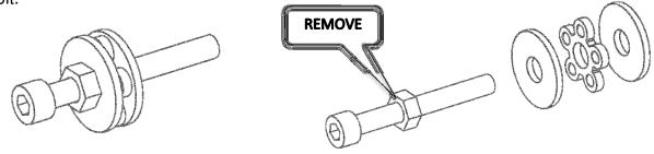
Replace the washers and bearing plate. Thread the bolt into a nutserts and tighten with a M6 allen wrench to set the nutserts. Torque the nutserts to the specification below to insure that they are set correctly.
