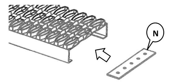
Align the strap brackets that were placed inside the board on the previous step with the braces that are attached to the vehicle (Braces B&C). Place an angle brace (O) on the brace board mounting area. Attach the running board to the brace using three bolts (L), six washers (I), and three nuts (J) at each location and repeat for all braces. Do not completely tighten the hardware at this time.
