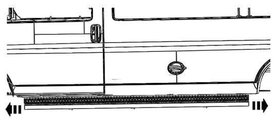
Once the board is in the proper location, clamp the running board to the braces.
