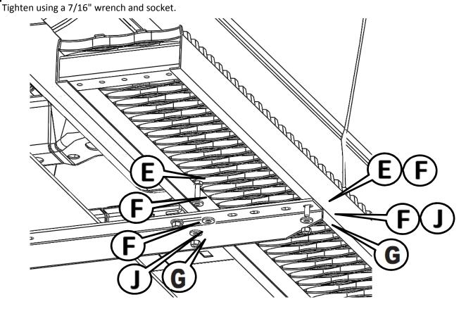
Check all hardware to make sure it has been tightened. Repeat the assembly steps for the other side of the vehicle.
