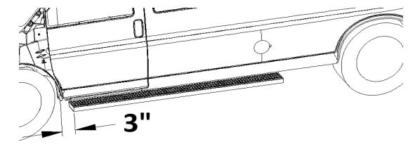
Once the board is in the proper location, clamp the running board to the angle braces.
