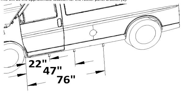
Make sure there is nothing on the frame at these three location that would obstruct the frame bracket from being installed in the later steps. If there is an obstruction, move the rocker panel bracket to the front/rear as needed.
