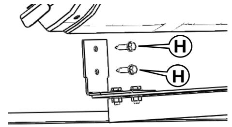
Remove the clamps holding the frame bracket [F] to the frame. Repeat this step for each bracket location.
