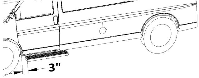
Once the board is in the proper location, clamp the running board to the angle braces.
