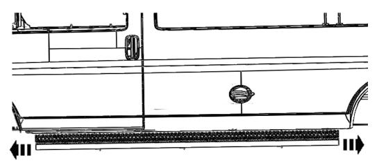
For the 155" wheel base van, set the board location 3" from the front wheel well.
