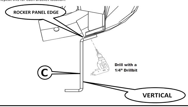
Attach the rocker brackets [C] to the rocker panel with a ribneck carriage bolt [I], washer [F], and nut [G].
