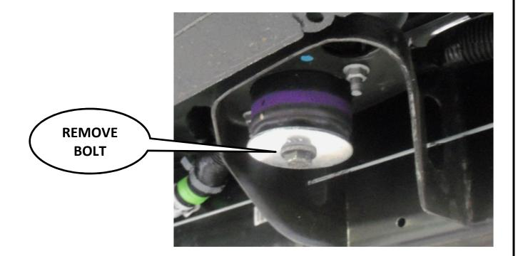
Put the body shock mount bolt through the hole in the brace and thread it back into the body shock mount. Align the braces so that they are perpendicular to the side of the vehicle. Tighten the bolts to 44 ft-lbs plus another half turn.
