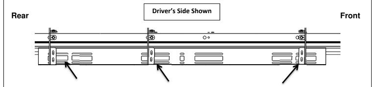
Remove the tube and install the 8mm U-nuts that came with the Step Tubes (J) into the slots identified above. Use 2 U-nuts per brace location. Repeat on other side
