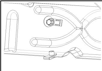
If your vehicle has the weld nut in the front and middle locations, thread the bolt part way into the weld nut.
