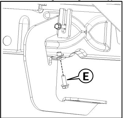
Tighten the 8mm bolts using a 13mm wrench.
