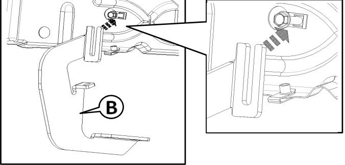
Attach the bottom mounting location using the 8mm bolt [E].
