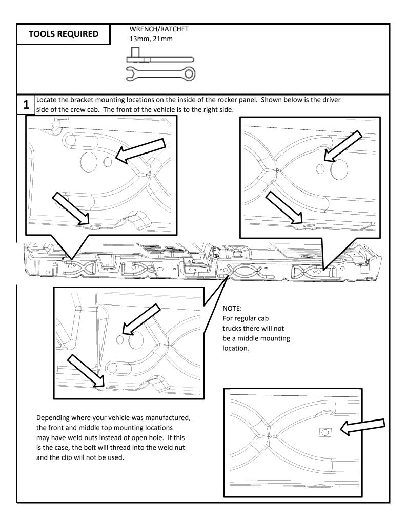
Install the 8mm U-nut [F] in all of the mounting locations, unless there is a weld nut.
