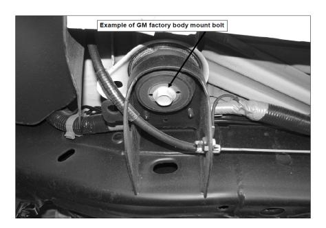
Using a 21mm socket, remove the front body shock mount bolt from the passenger side.
