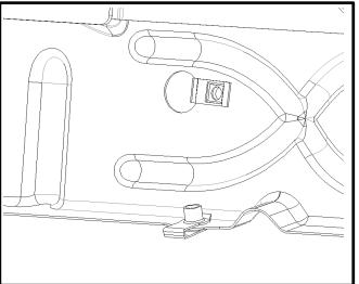
Thread an 8mm bolt [E] part way into all of the top mounting locations.
