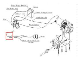
2) Secondly, cut the connector of receiver.
