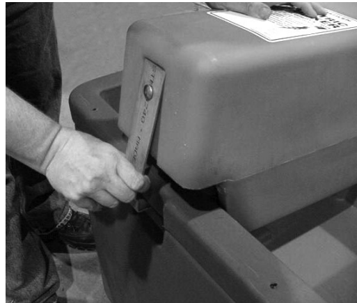
Illustration # 3A - Pull on Latch Handles
