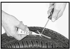
Remove a plug from its clear backing, then thread it halfway through the eye of the plugger needle. Coat the middle section of the tire plug with Plug Bond.
