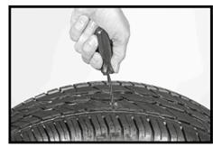
Slide the reamer tool in and out of your tire puncture multiple times to roughen and clean the inside of the hole.
