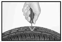
With the plug centered in the eye of the needle, start pushing the plugger tool and plug into your puncture. Stop pushing when the plug is 2/3 of the way into the hole.
