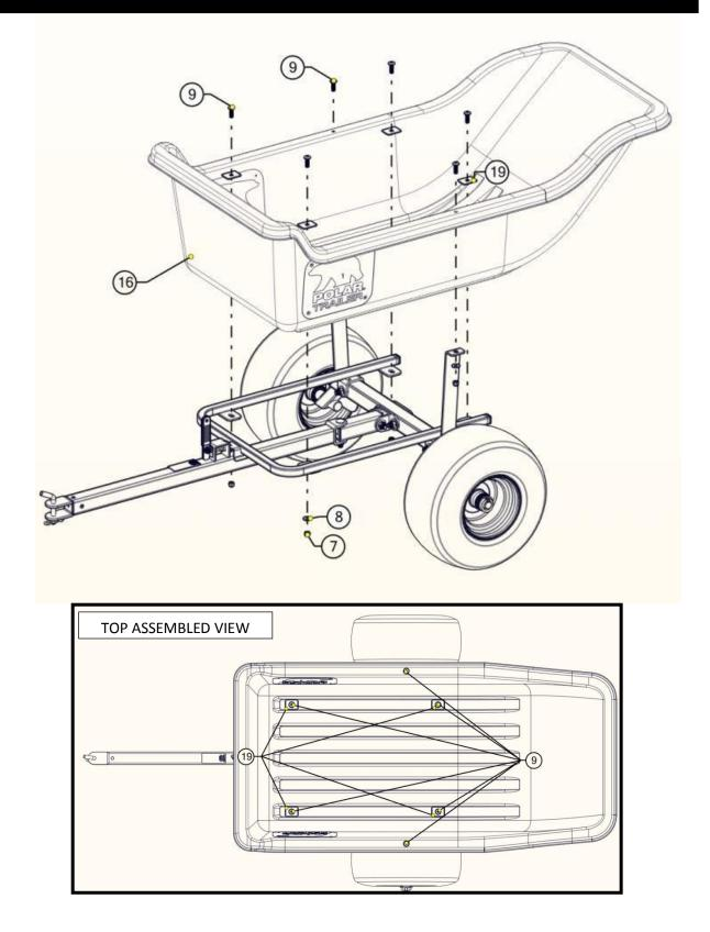
At this point tighten all of the nuts and bolts to finish the assembly process.
