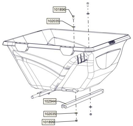
1. POSITION 102957 (BOTTOM HANDLE) IN PLACE AS SHOWN AND ASSEMBLE TO 102944 (HANDLE BRACKET) AS SHOWN. FOLLOW SAME PROCESS FOR OTHER SIDE.
