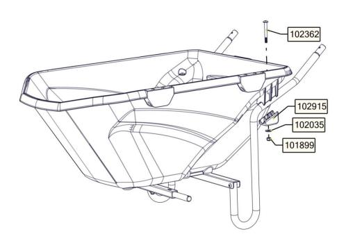
1. PUSH 102958(TOP HANDLE) INTO PLACE OVER BOTTOM HANDLES AND ASSEMBLY AS SHOWN.
